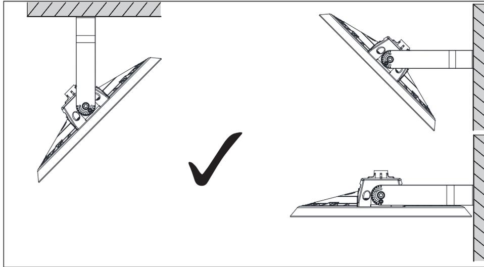
*For all of the above installation, it is recommended that all models with safety rope.*
